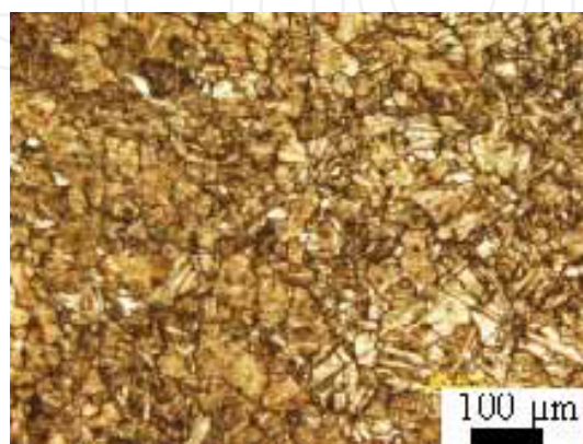
Fig. 1-1. Optical microstructure of as-received extrusion AZ31 magnesium alloys used.
