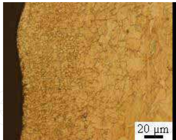
Fig. 3-5. Sub micron size microstructure at surface of AZ31 Mg alloy by MAF work, hydrogen treatment and shot penning with recrystallization treatment.
