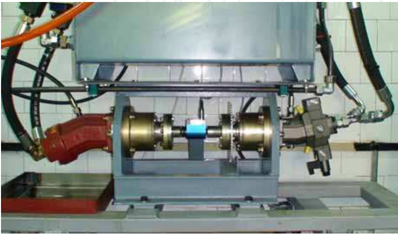
Fig. 12. Bosch servo motor, type EP2, within the secondary sector
