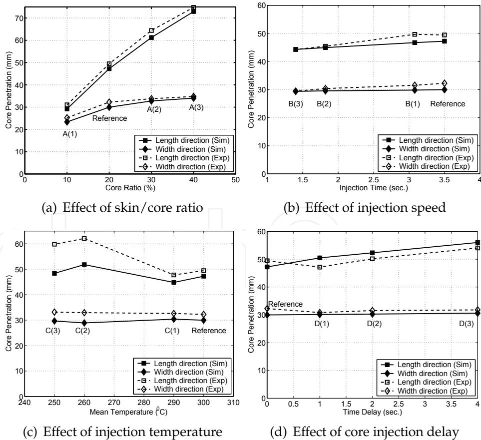
Fig. 5. Comparison of numerical and experimental core penetration
