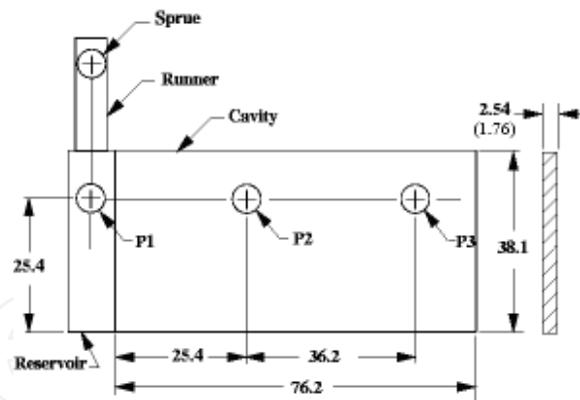
Fig. 1. Geometry of the cavity and location of control points P1, P2 and P3
