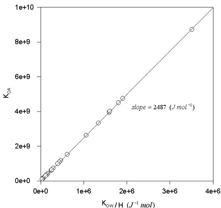
Fig. 7. Calculated  $K_{OA}$  (eqn. 2) vs ( $K_{OW}/H$ )
