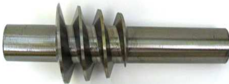
Fig. 20. A grinded Archimedean spiroid worm with cylindrical foot surface
