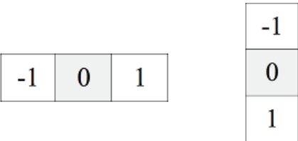
Fig. 1. Gradient kernel in horizontal direction on the left and vertical direction on the right. Kernel center is marked with grey color.
