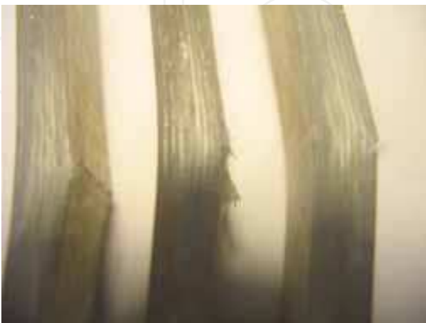
Fig. 33. Failure area of some specimens reinforced only with E-glass fibres, after flexural test
