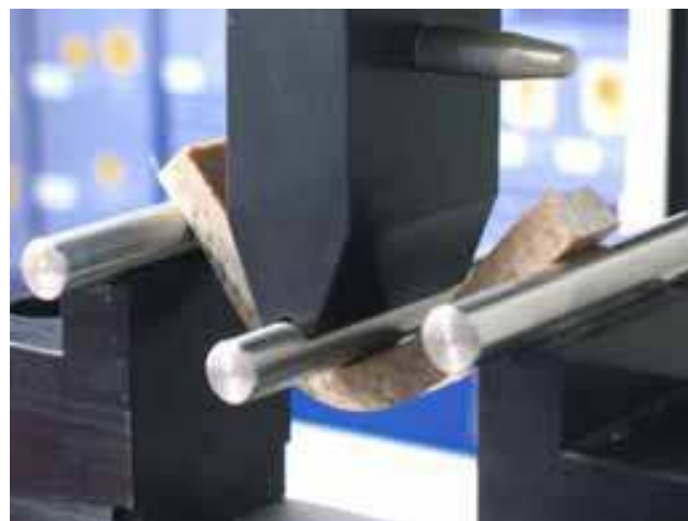
Fig. 5. Specimen made of E-glass EWR145 / oak wood flour / polyester Colpoly 7233 during flexural test
