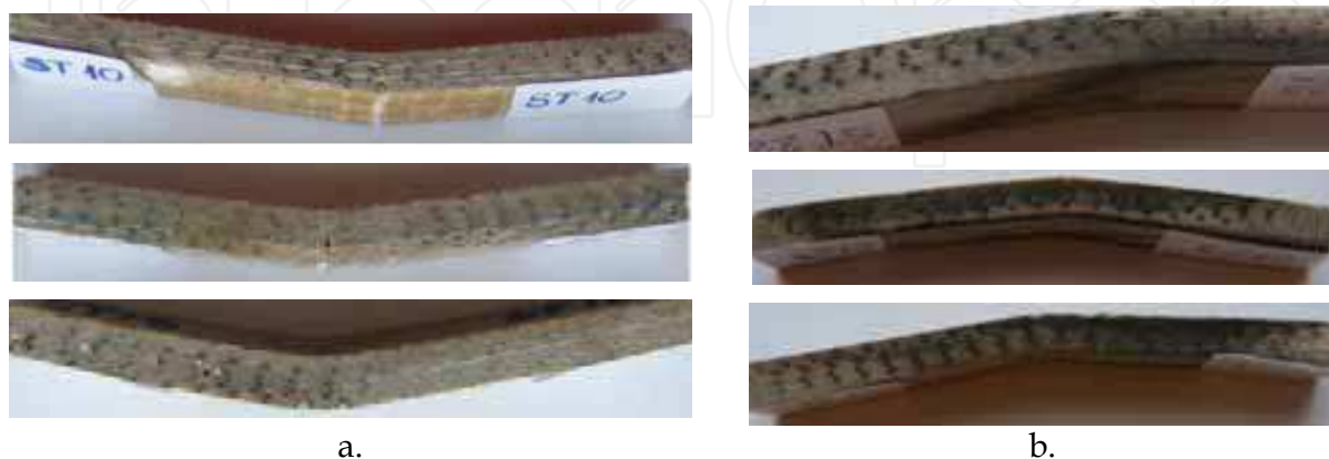
Fig. 37. Photos of the edges of the specimens made of E-glass / oak wood flour / polyester after 5853 hours of immersion in: a) water; b) seawater
