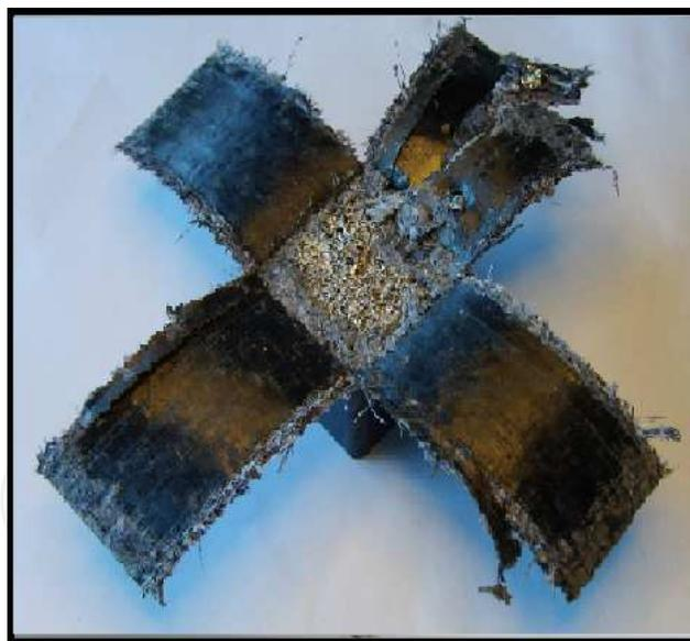
Fig. 16. Crush pattern of foam-filled composite crash box
