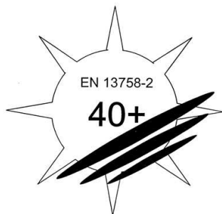
Fig. 1. Pictogram for UV protective clothing according to the EN standard 13758-2
