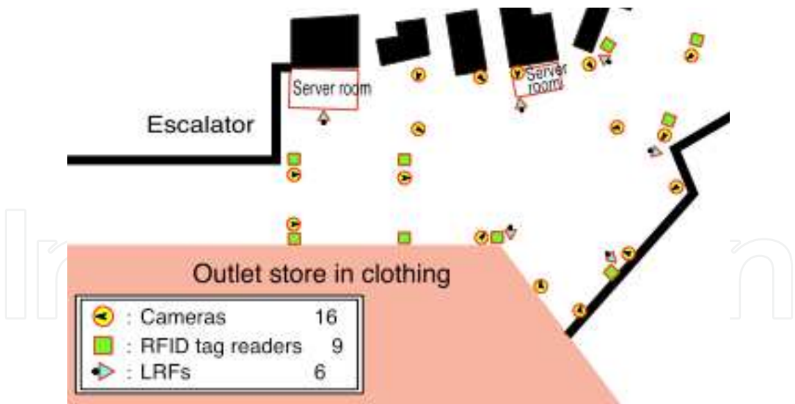
Fig. 8. Sensor alignments in the Kansai Environment (UCW).
