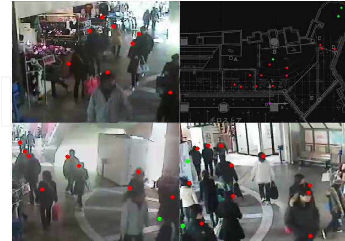
Fig. 6. Example of the integrated position estimation. The red dots show the head estimation results and the green dots show the torso estimation where head was not detected or when person was out of camera tracking area.
