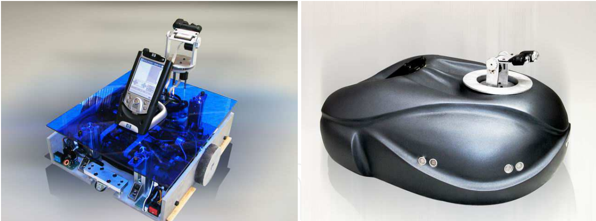
Fig. 8. Shape of the PBMoRo (Left image) before considering robot design, (Right image) after adapting robot design.
