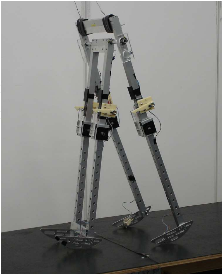
Fig. 8. Walker on the ramp, outfitted with knees with active release system.
