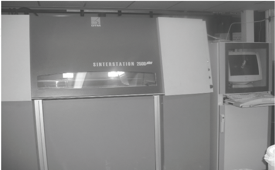
Fig. 4. The SLS Sintersation 2000 apparatus (Courtesy of CRDM)
