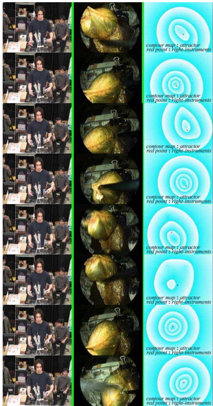
Fig. 8. View of an in vitro experiment (laparoscopic cholecystectomy) using a swine liver with a gallbladder (4/6). (left) a surgeon and the laparoscope robot P-arm, (mid) image from the laparoscope, (right) visualization of attractors as the contour map on the image plane.
