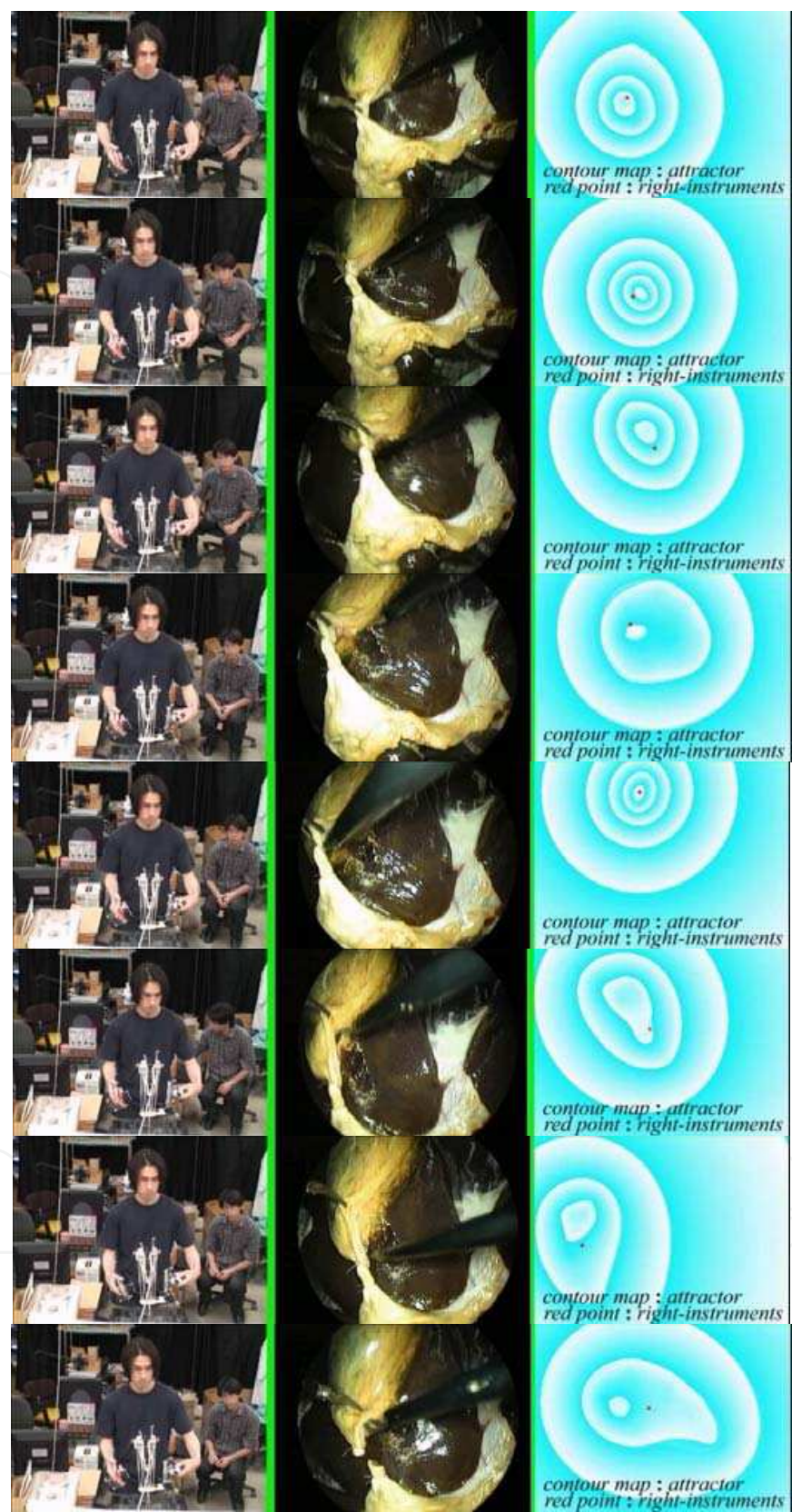
Fig. 5. View of an in vitro experiment (laparoscopic cholecystectomy) using a swine liver with a gallbladder (1/6). (left) a surgeon and the laparoscope robot P-arm, (mid) image from the laparoscope, (right) visualization of attractors as the contour map on the image plane.
