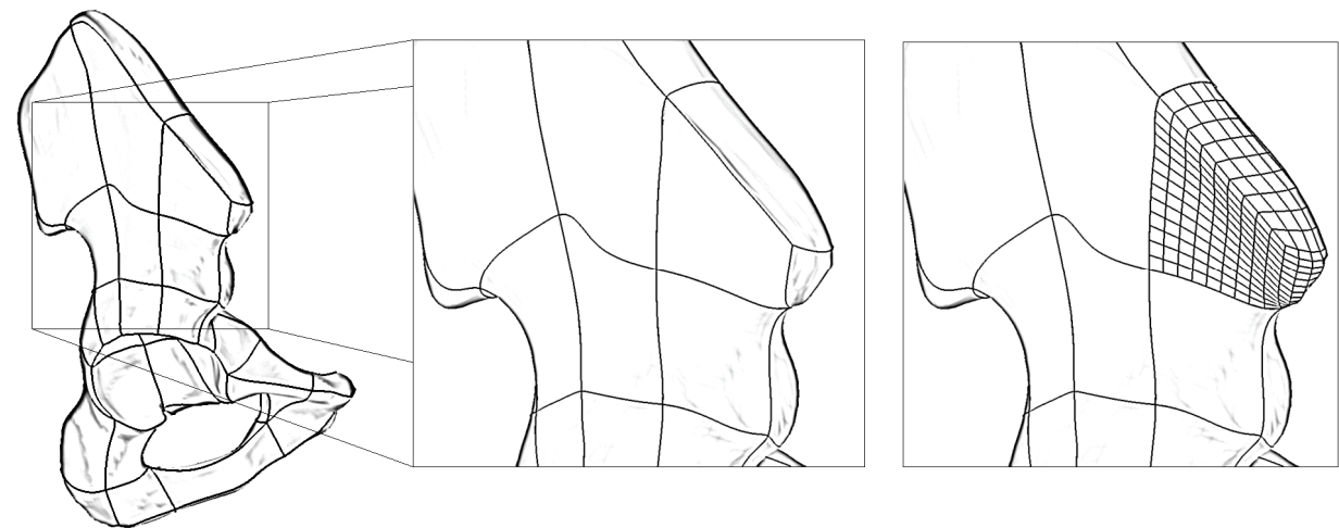
Fig. 5. Distribution of NURBS-surfaces such that quadrilateral surfaces are oppositely located enables generation of solids with five or six faces. Such solids can be meshed with hexahedral elements automatically.
