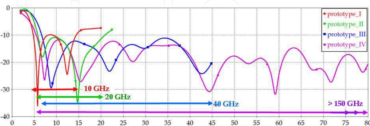
Fig. 5. Impedance bandwidth of the developed prototypes. Ordinate: magnitude of the reflection coefficient [dB]; Abscissa: frequency [GHz].
