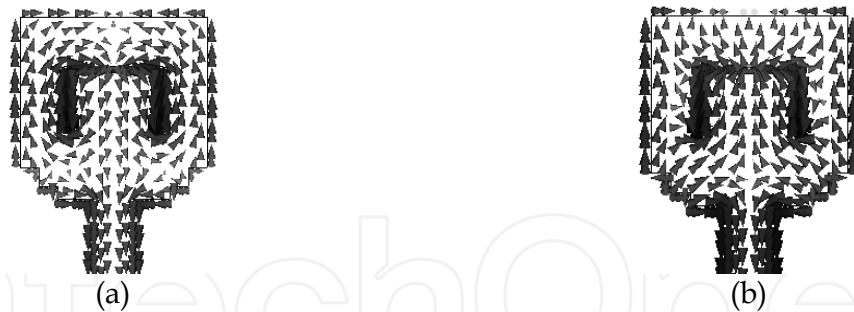
Fig. 7. Simulated current distributions. (a) 5.5GHz. (b) 7GHz.
