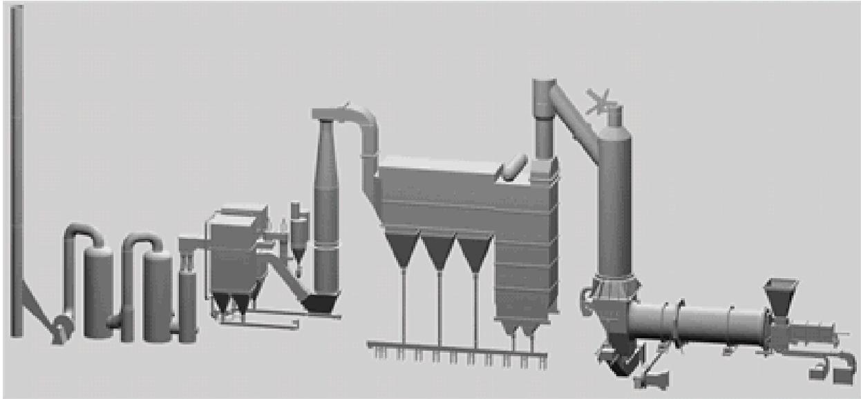
Fig. 7. Schematics of a rotary kiln incinerator
