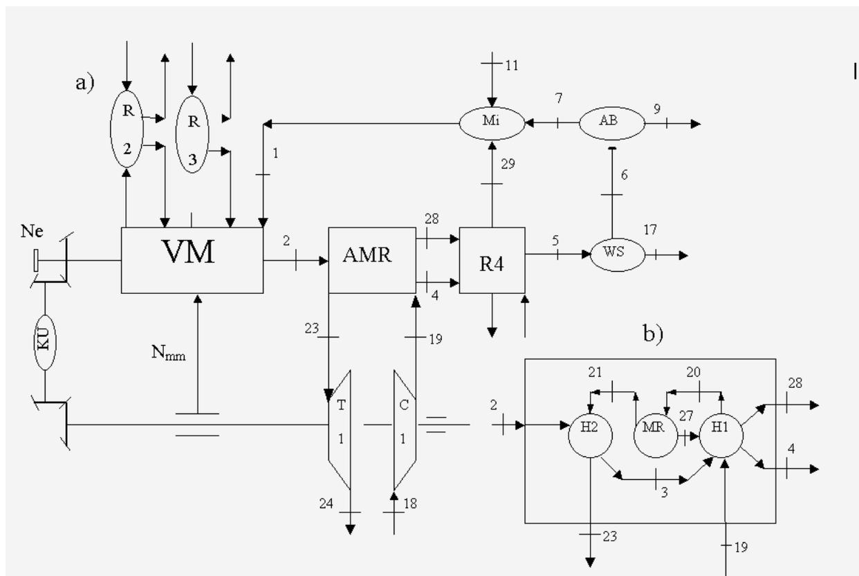
Fig. 2. Schematic of the ZEMPES with oxygen enrichment of an "artificial air" (O<sub>2</sub> + CO<sub>2</sub>).
