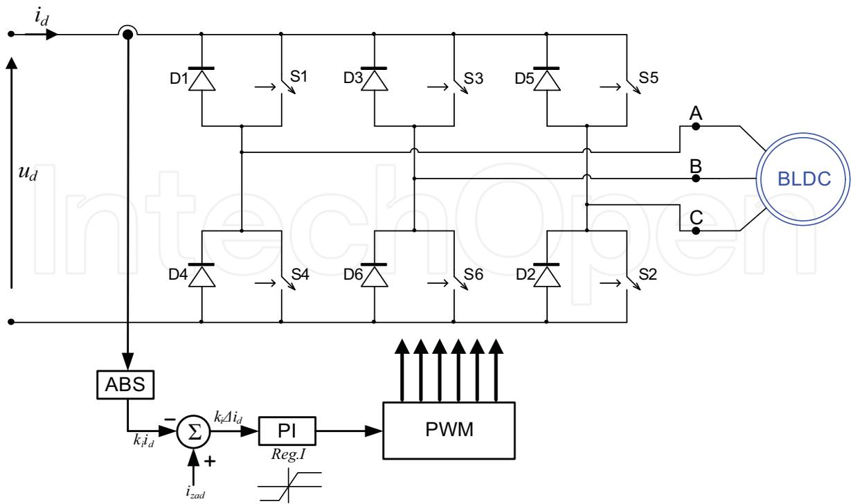
Fig. 10. Measurement of the inverter input current
