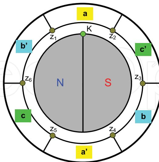
Fig. 12. The cross section of a BLDCM motor
