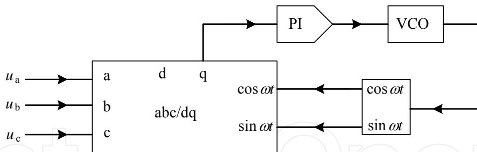
Fig. 16. Block diagram of the synchronization circuit
