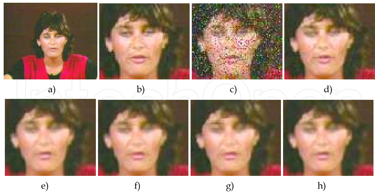
Fig. 3. a) 10 th Miss America original image, b) Zoomed region analyzed, c) 15% of impulsive noise, d) Proposal 3D-FD filter, e) 3D-MF; f) 3D-VMF, g) 3D-GVDF, h) 3D-VATM.
