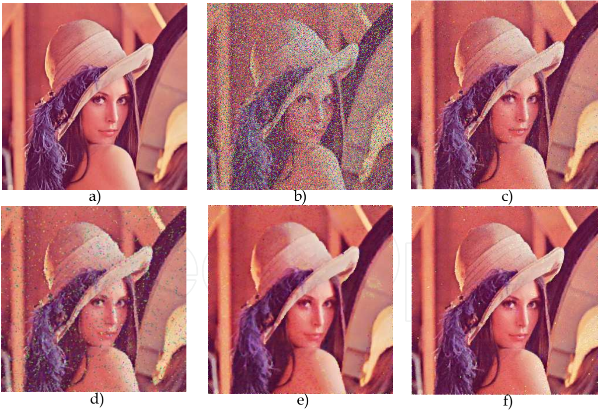
Fig. 5. Subjective visual qualities of restored colour image “Lena”, (a) Original test image “Lena”, (b) Input noisy image (with 20% of impulsive noise), (c) FASVM filtering image, (d) VMMKNN filtered image, (e) Proposed VMML filtering image (S,E,ND), and (f) Proposed VMML filtering image (S,E,D).
