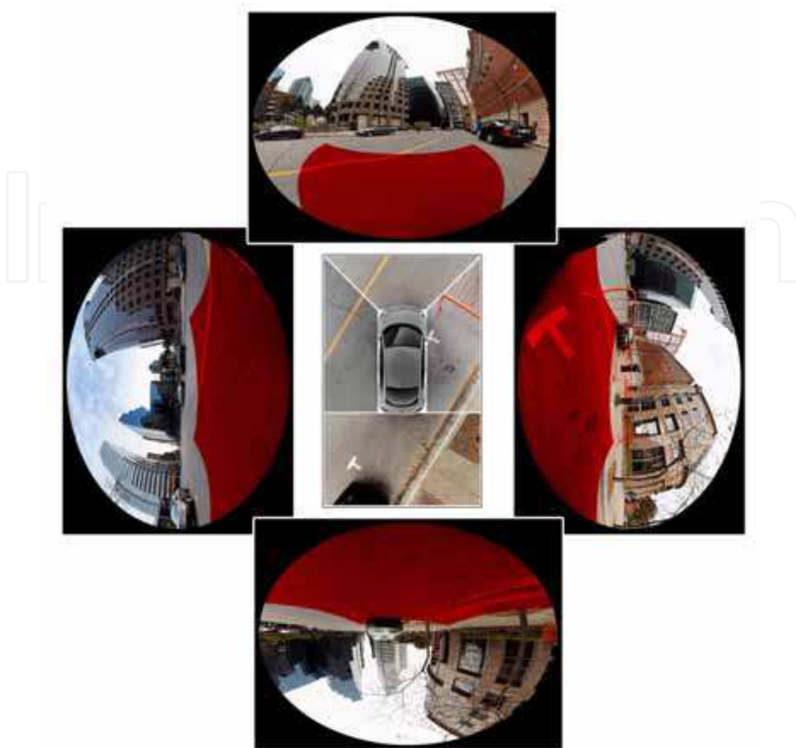
Fig. 31. View of area surrounding vehicle using four (4) panomorph lenses.
