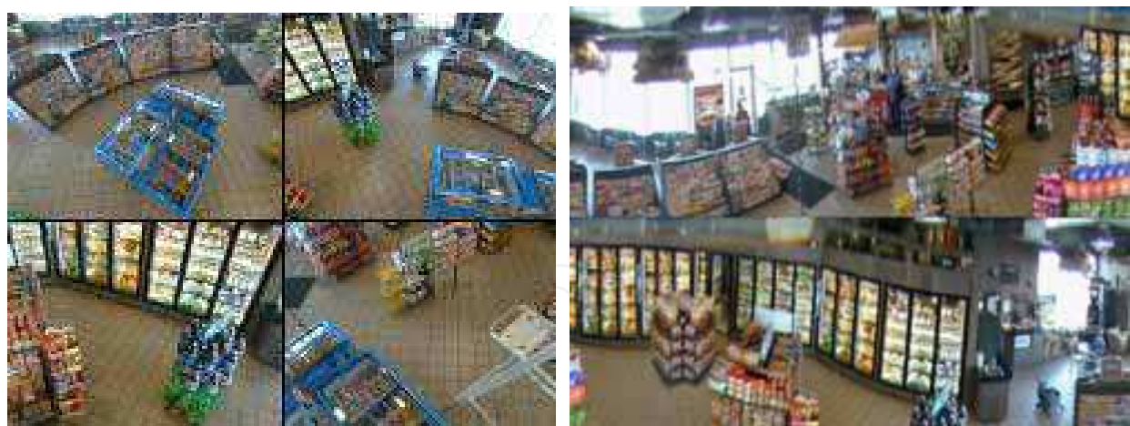
Fig. 9. Four PTZ views (left), and two strips to display a 360° total camera surround in one single view (right).
