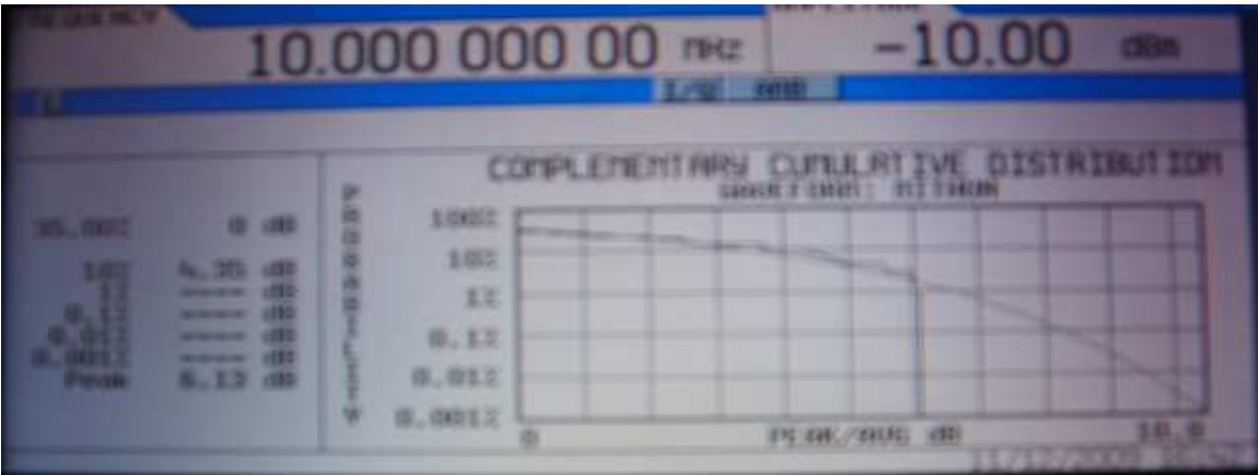
Fig. 10. CCDF of PAPR in 8-ary PSK for N=24 after code and phase optimization
