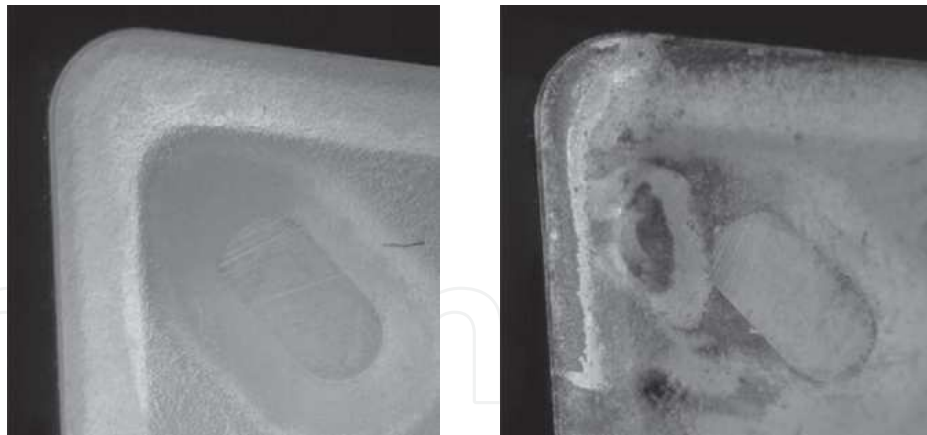
Fig. 4. Test surfaces: (left) new cutting insert; (right) worn cutting insert. The shown images were recorded with diffuse illumination (just for visualization purposes).
