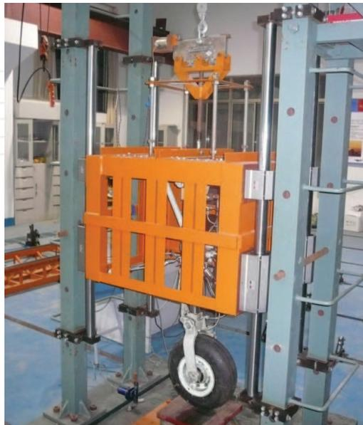
Fig. 7. Landing gear experiment platform
