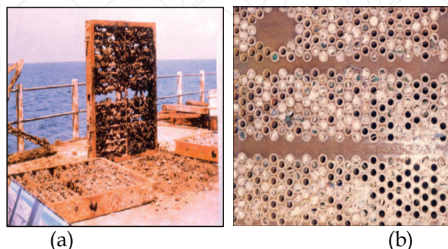
Fig. 4. Blockage of intake screen by fouling organisms (a) and blockage of condenser tubes by green mussels & barnacles (b)
