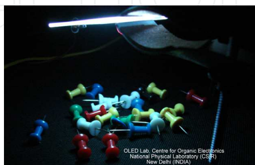
Fig. 2. 1"x1" proto type of a multilayer phosphorescent efficient WOLED developed at National Physical Laboratory, New Delhi, India
