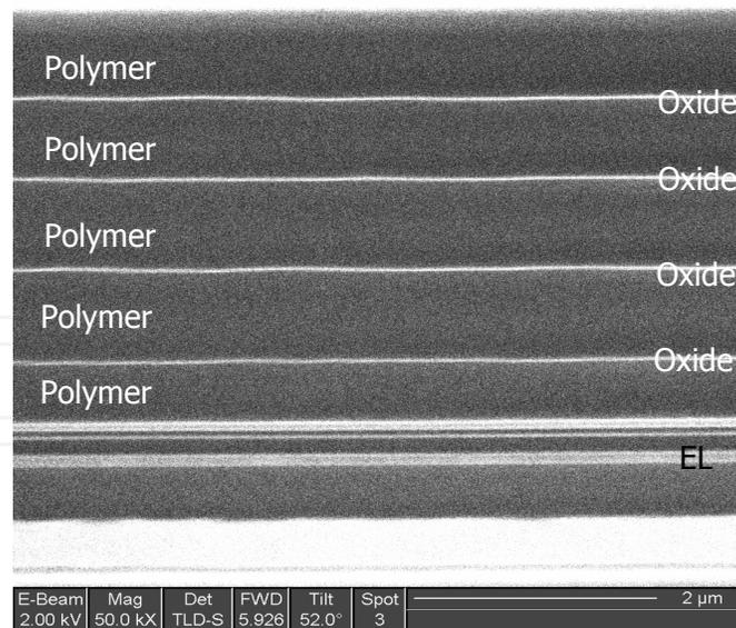
Fig. 29. SEM image of thin film encapsulated AMOLED.
