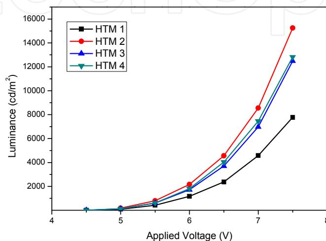
Fig. 6. Luminance-applied voltage characteristics of devices III-VI.
