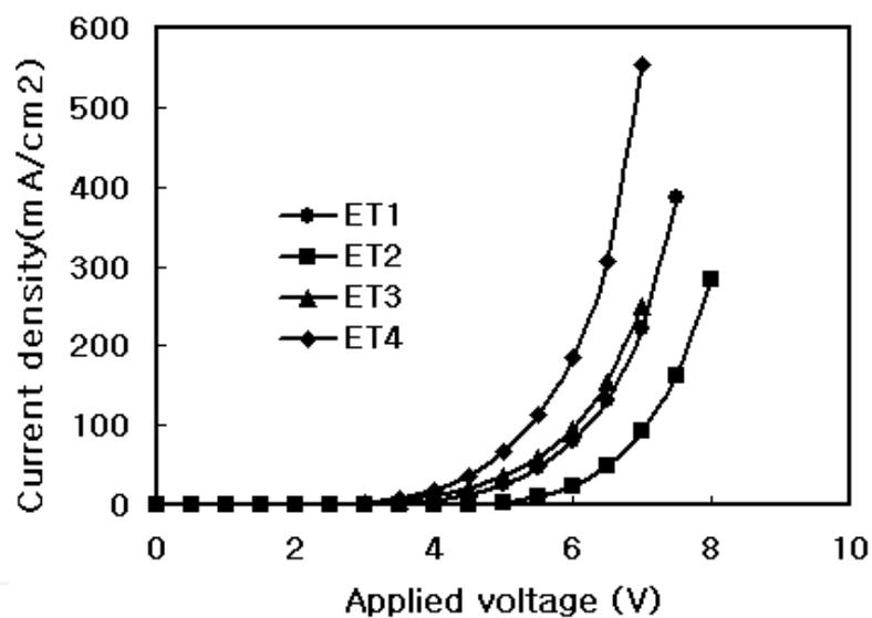
Fig. 12. Voltage-Current curve of ADN series ETMs
