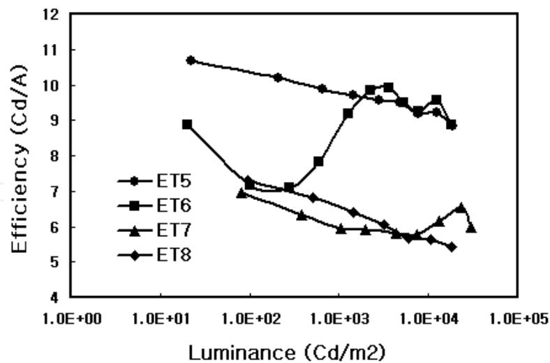
Fig. 15. Luminance-Current efficiency curve of Phenanthroline series ETMs
