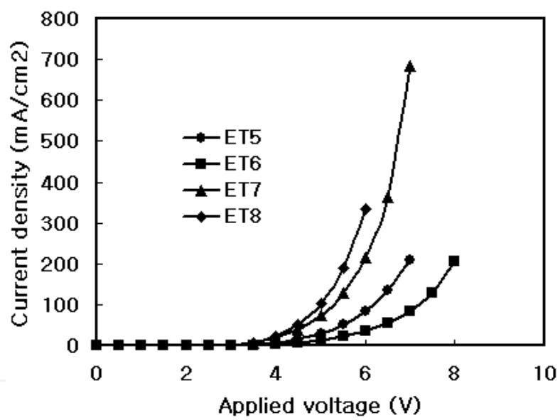
Fig. 14. Voltage-Current curve of Phenanthroline series ETMs
