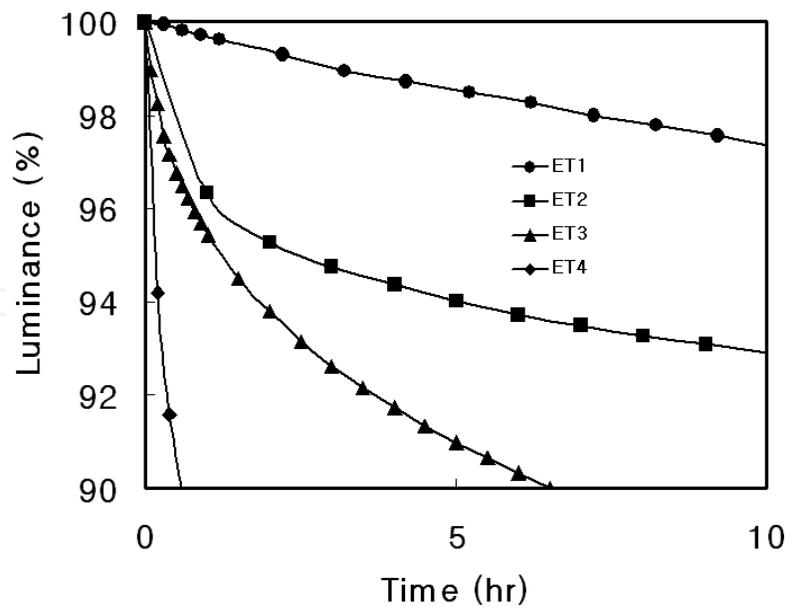
Fig. 16. Initial luminance decrease tendency of devices with ADN series ETMs at 100mA/cm<sup>2</sup>.
