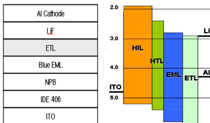
Fig. 11. Blue OLED structure and Energy diagram
