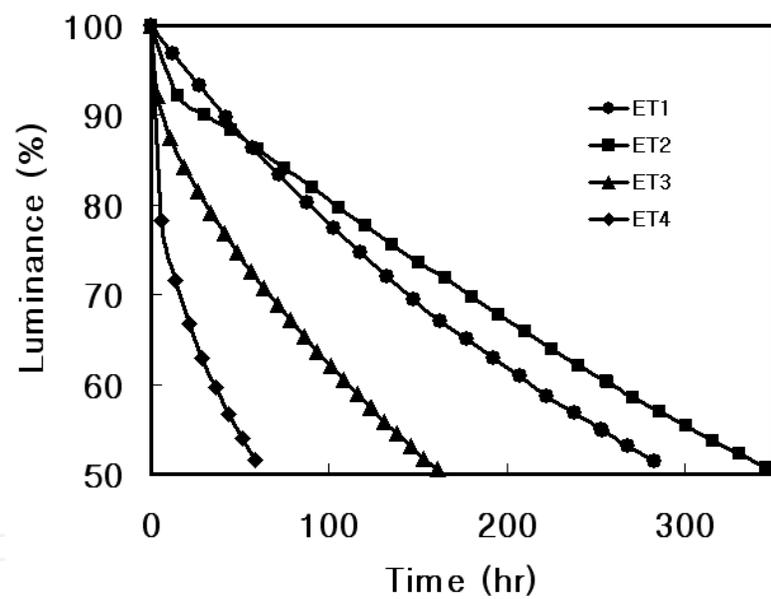
Fig. 16. Life time (half-life) tendency of devices with ADN series ETMs at 100mA/cm<sup>2</sup>
