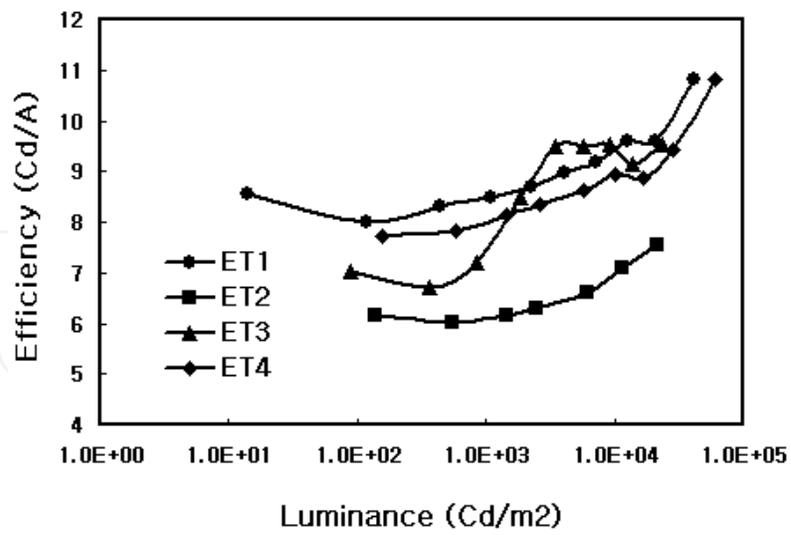
Fig. 13. Luminance-Current efficiency curve of ADN series ETMs
