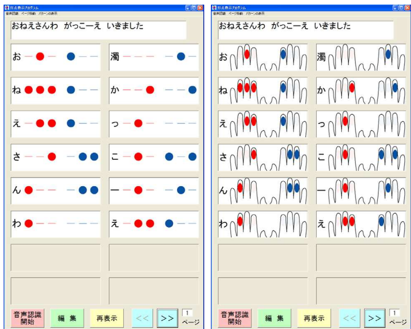
Fig. 15. Expanded teaching interface, presentation method A (left) and B (right). Displayed dot pattern is “Oneesanwa / gakko-e {My sister / to school.}”
