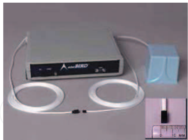
Fig. 12. MiniBIRD 6 DOF magnetic sensor
