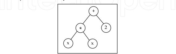
Fig. 1. Sintax tree for  $(x^*x+2)$
