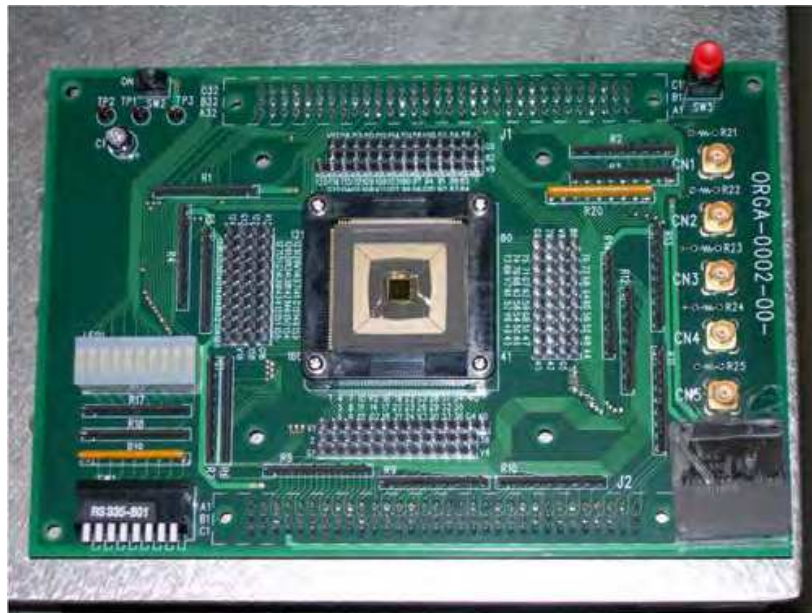
Fig. 3. Photograph of an ORGA-VLSI board with a fabricated ORGA-VLSI chip. The ORGA-VLSI was fabricated using a 0.35\ \mu\text{m} three-metal 4.9 \times 4.9\ \text{mm}^2 CMOS process chip. The gate count of a gate array on the chip is 68. In all, 340 photodiodes are used for optical configurations.
