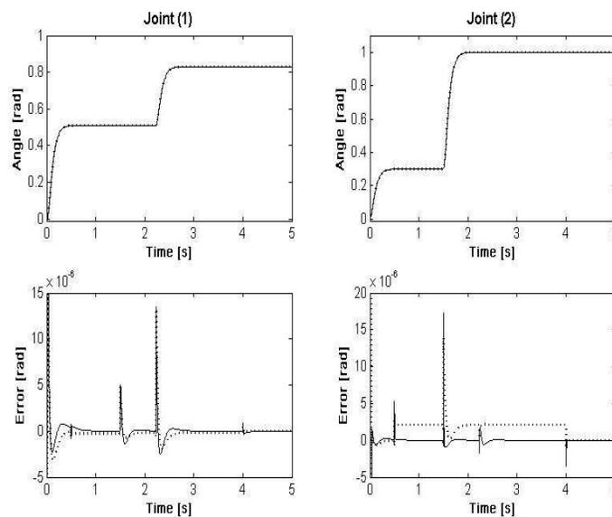
Fig. 5. Angular positions and tracking errors of distributed system with uncertainties compensator. .... reference, -.-.- estimate with compensator (45), — estimate with compensator (49) ..... tracking error with compensator (45), — tracking error with compensator (49)
