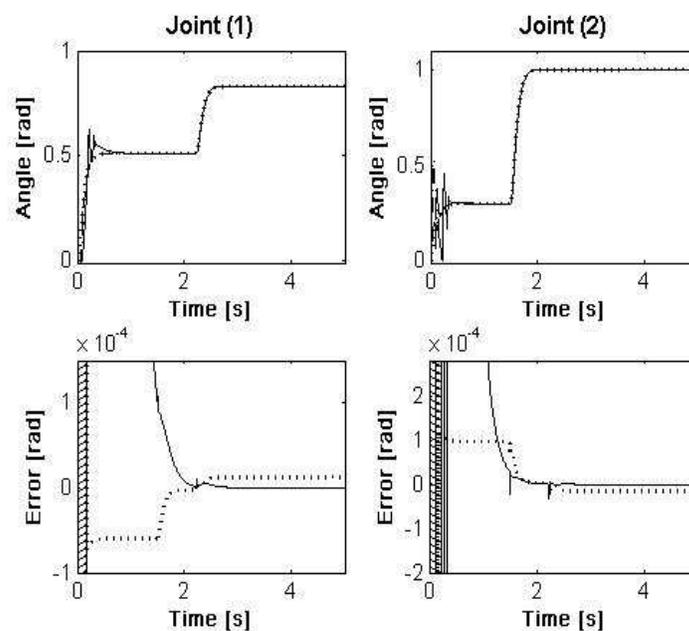
Fig. 7. Angular positions and tracking errors of mismatched model with uncertainties compensator. .... reference, - · - · - estimate with compensator (45), — estimate with compensator (49). .... tracking error with compensator (45), — tracking error with compensator (49)
