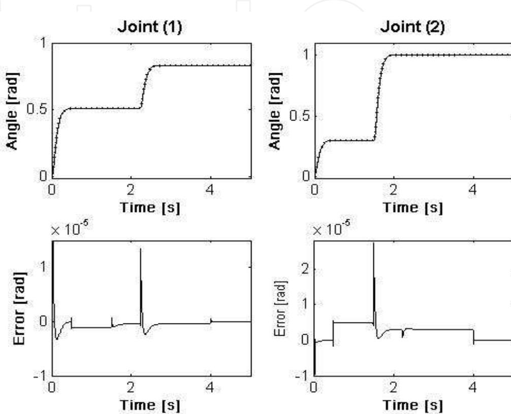
Fig. 2. Angular positions and tracking errors of distributed system without uncertainties compensator. .... reference, ——estimate
