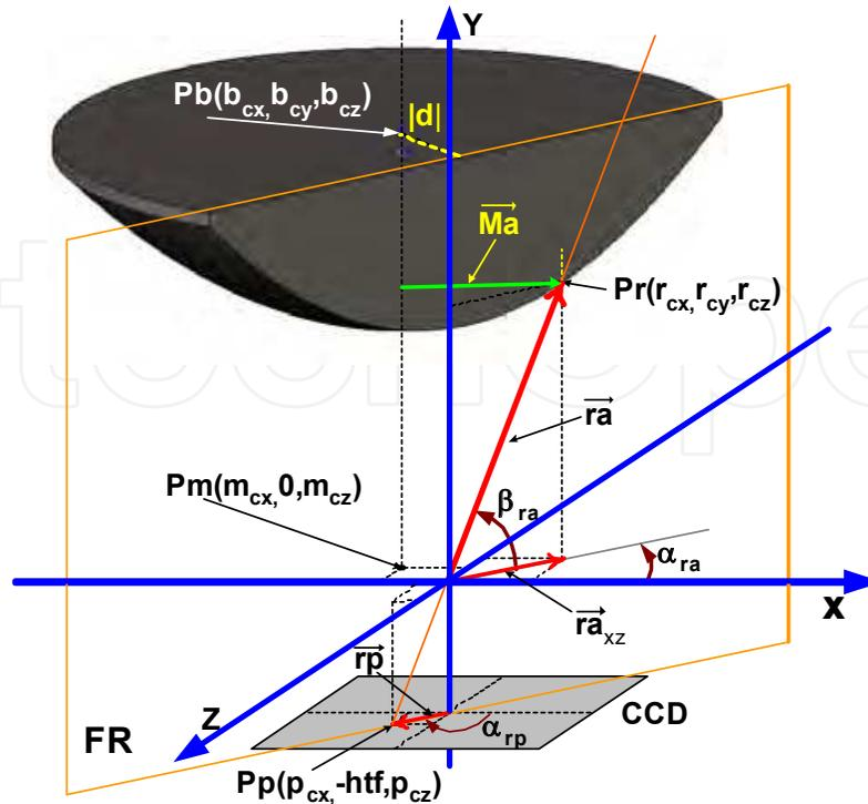
Fig. 6. A random pixel in the CCD sensor plane is the start point for the back propagation ray. This ray and the Y axis form a plane,  $FR$ , that intersects vertically the mirror solid.  $Pr$  is the intersection point between  $ra$  and the mirror surface.
