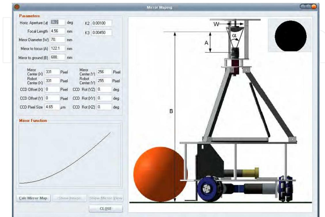
Fig. 11. Obtaining the pixel distance mapping on the ground plane; application interface.
