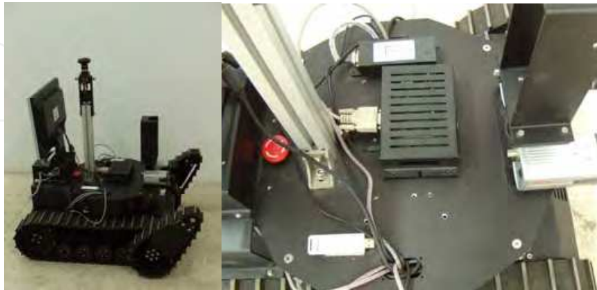
Fig. 12. fish-eye lens camera and embedded image processor
