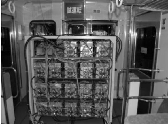
Lithium ion battery for VVVF type railcar
