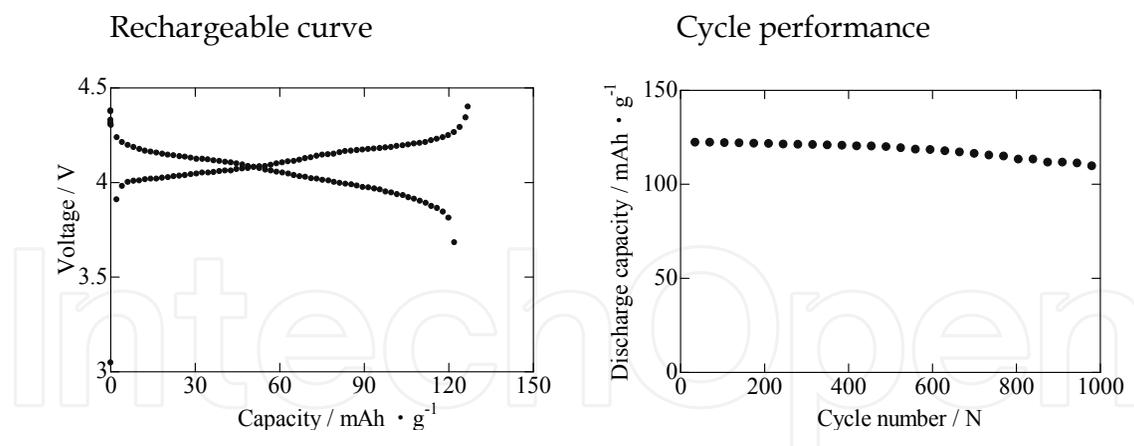
Fig. 3. Rechargeable curve and cycle performance of cathode
