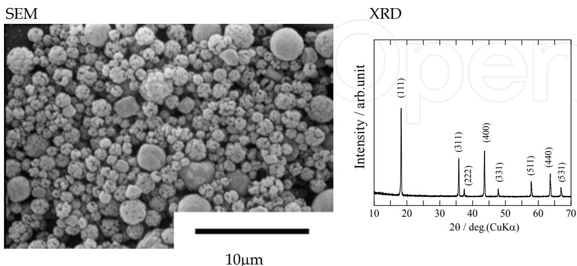
Fig. 2. SEM photograph and XRD pattern of LMP
