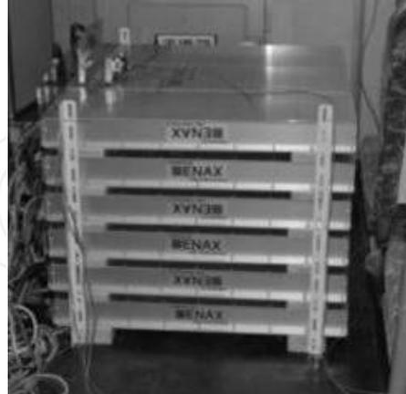
Fig. 4. Lithium ion battery module for railcar
