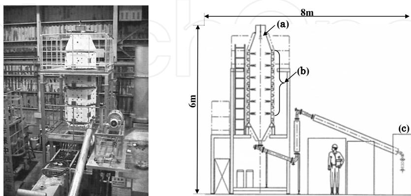
Fig. 1. Flame type spray pyrolysis apparatus
