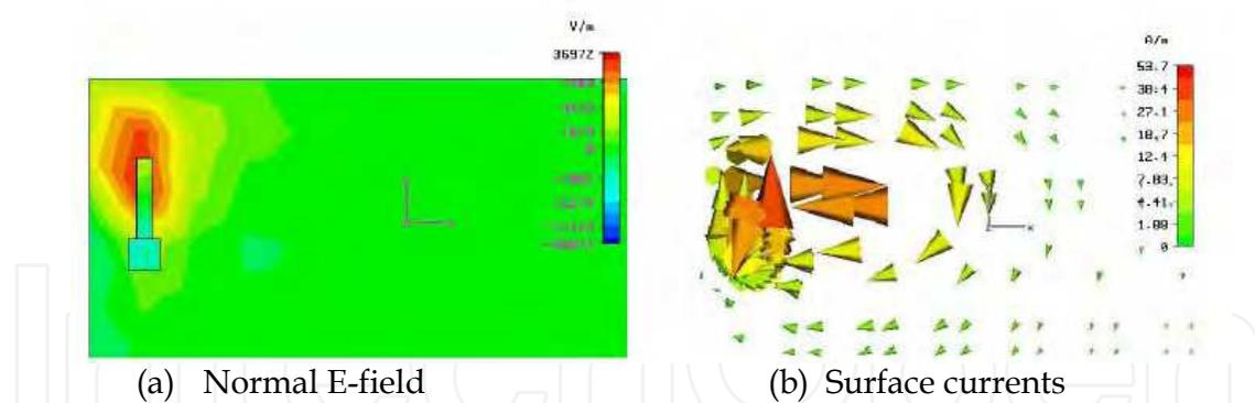
Fig. 17. The field distribution of proposed antenna
