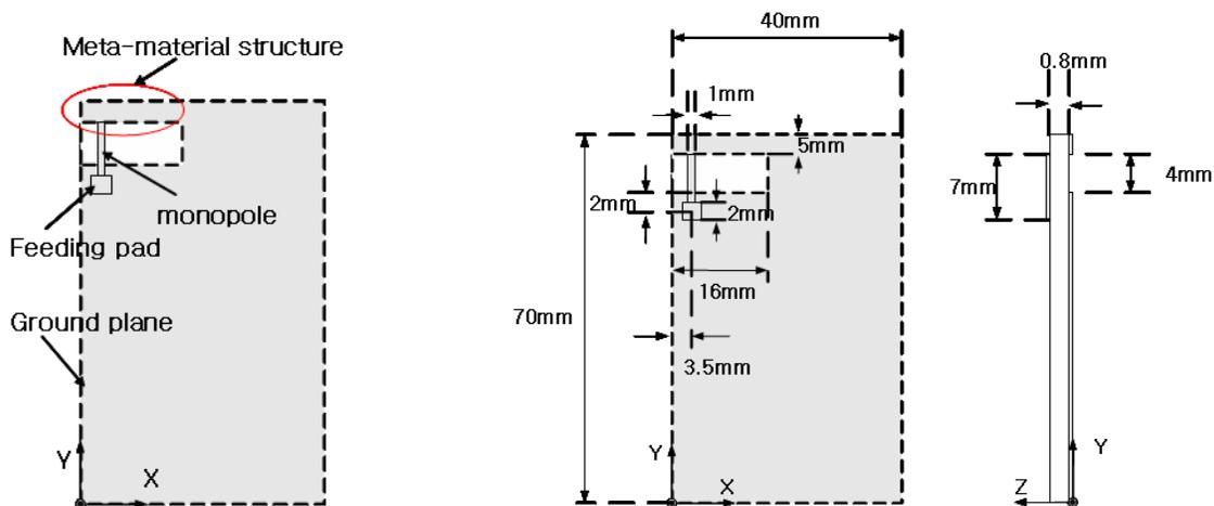
(a) The idea of proposed antenna (b) The geometry of proposed antenna
