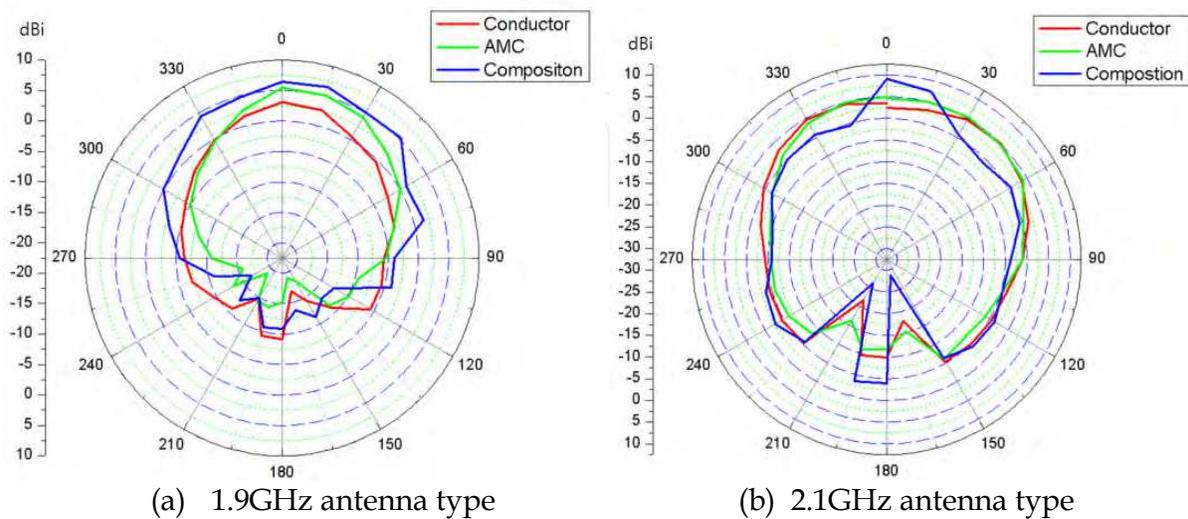
Fig. 39. The measured radiation patterns against antenna types
