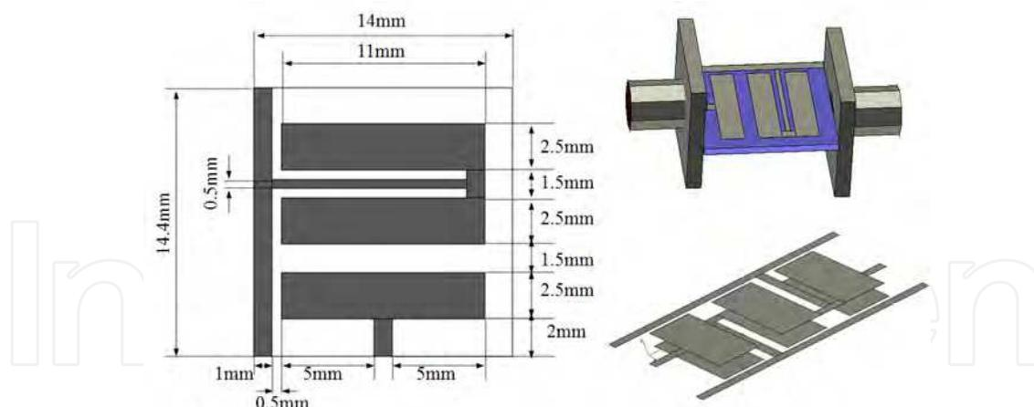
Fig. 8. The geometry of proposed NPLH transmission line
