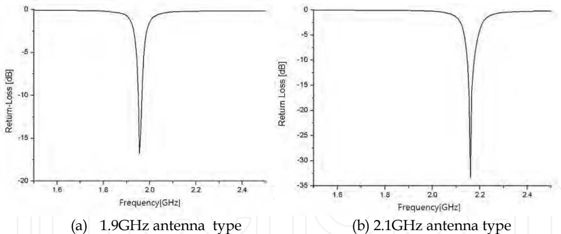
Fig. 38. The measured return-loss against antenna types
