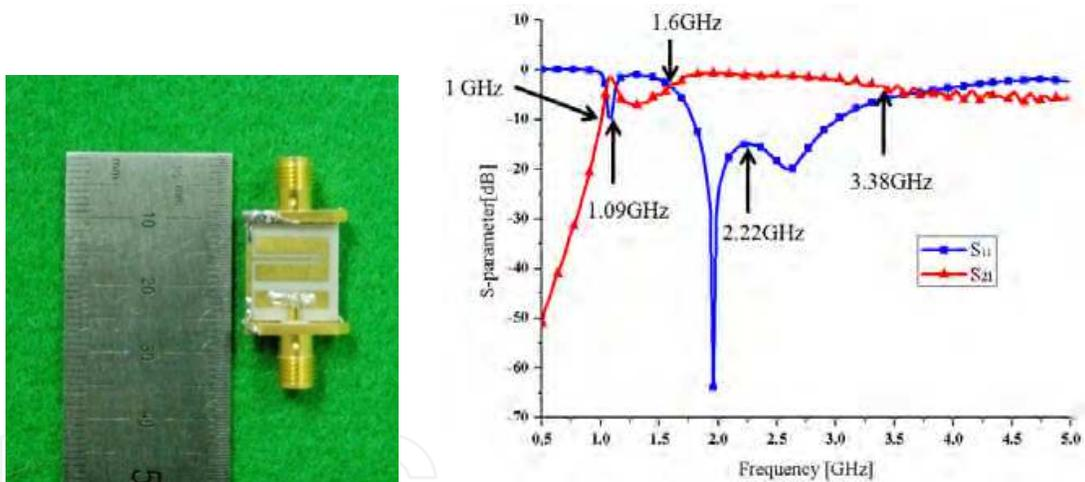
(a) The photo of NPLH transmission line (b) The measured S-parameter
