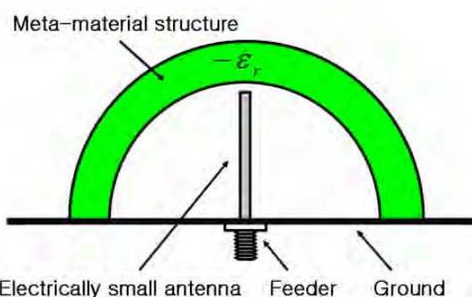
Fig. 13. The concept of proposed antenna
