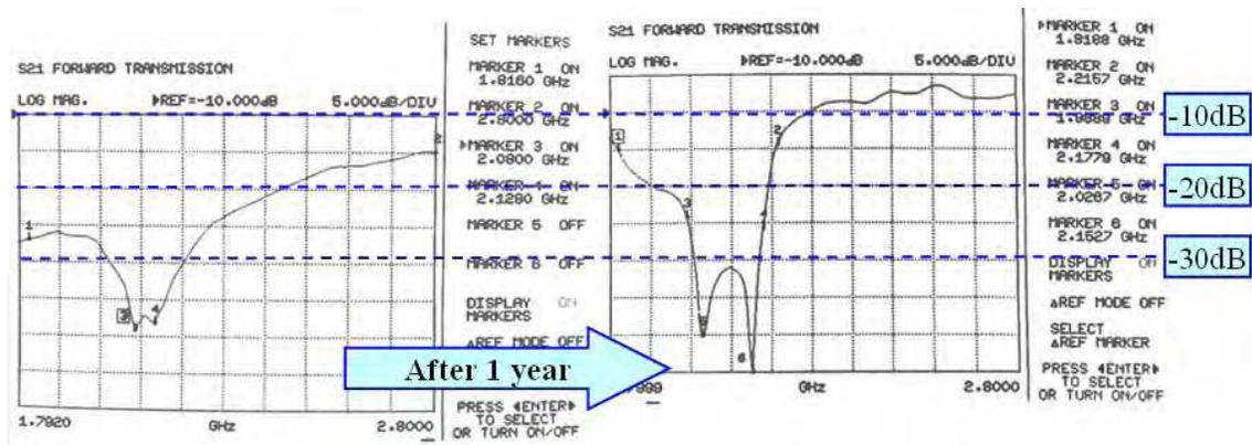
(b) Transmission coefficient of concrete block including 2 kinds of resonators
