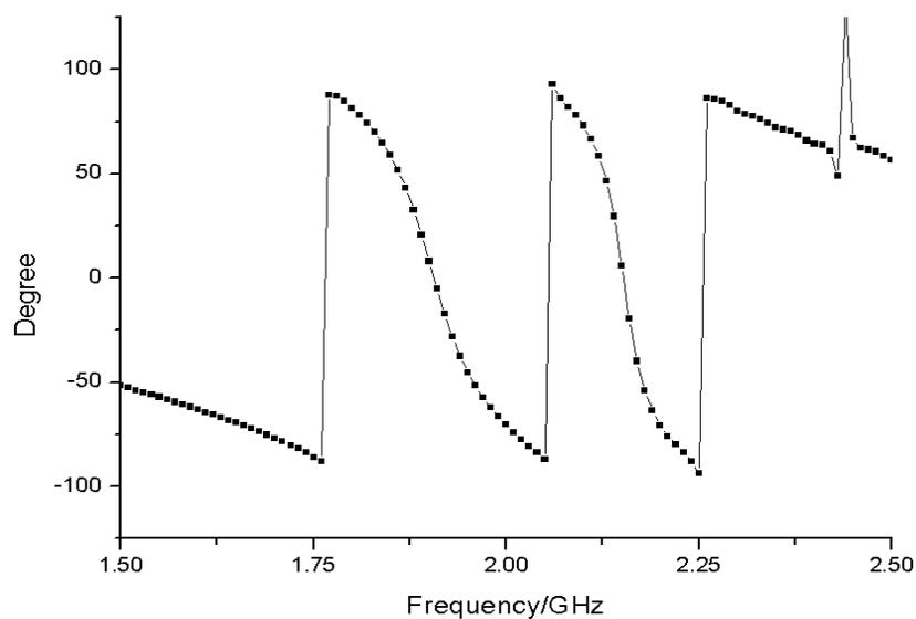
Fig. 32. The phase of proposed dual-band AMC structure
