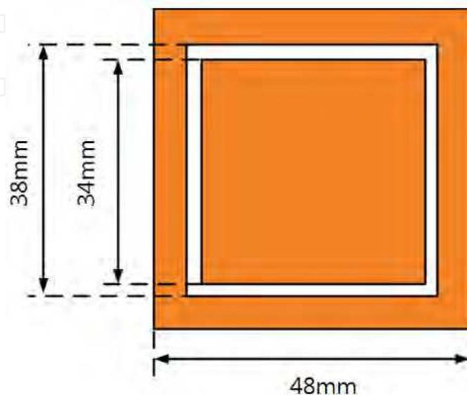
Fig. 23. The unit cell of FSS structure
