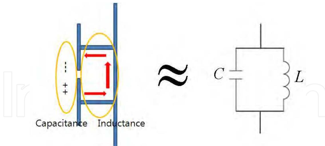
Fig. 27. The mushroom structure and equivalent circuit
