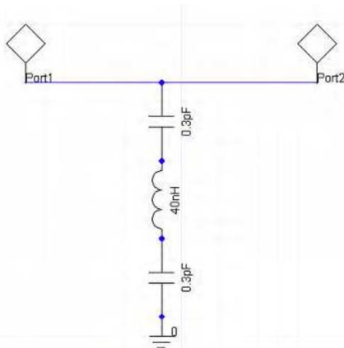
(a) Equivalent circuit of unit cell
