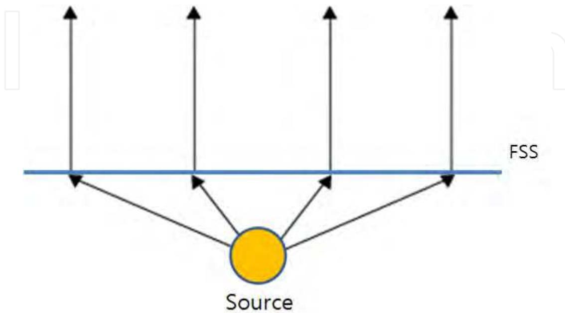
Fig. 21. The concept of lens using FSS structure
