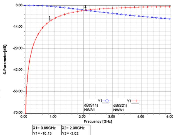
Fig. 4. The S-parameter of PLH transmission line circuit
