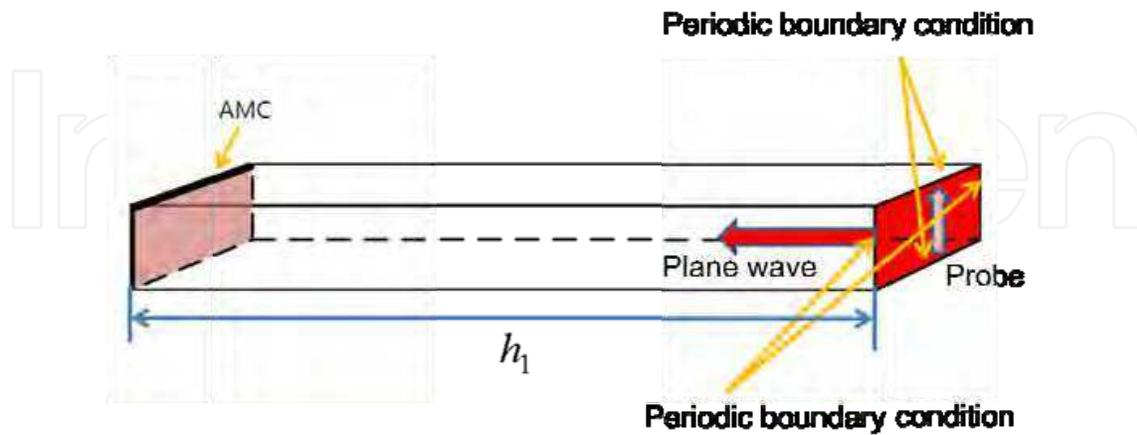
Fig. 29. The proposed analysis method of AMC
