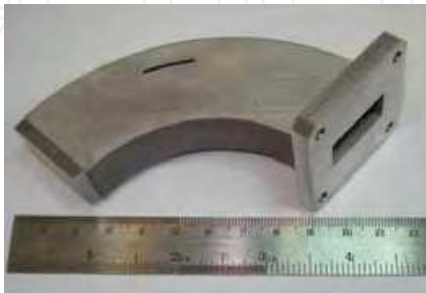
Fig. 8 The implemented AWSA structure: It is implemented through exact aluminum wire-cut procedure of each face and final assembly step. (Ebadi et al., a, 2007)
