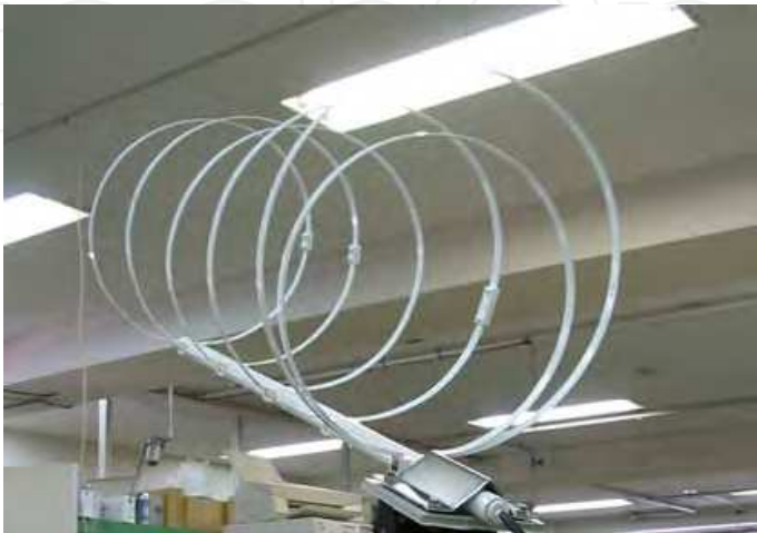
Photo 2.Right-hand Circularly Polarized Ring Loop Antenna
