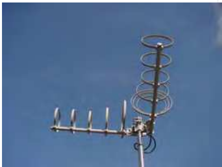
Photo 5. pattern synthesis of ring loop antenna
