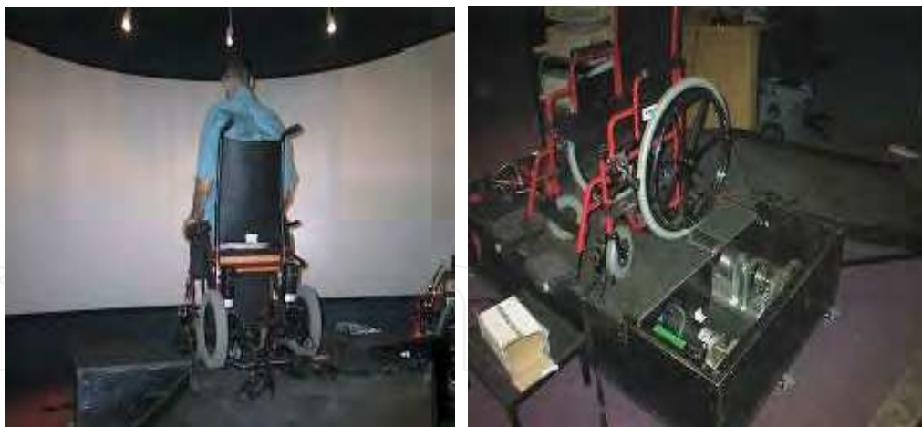
Fig. 11. Simulation platform for manual and electric wheelchair
