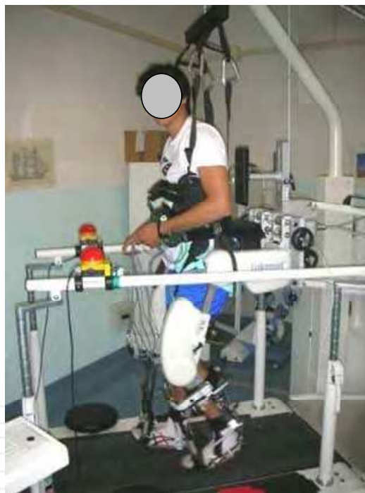
Fig. 4. The “Lokomat” robotic system for the lower limbs rehabilitation
