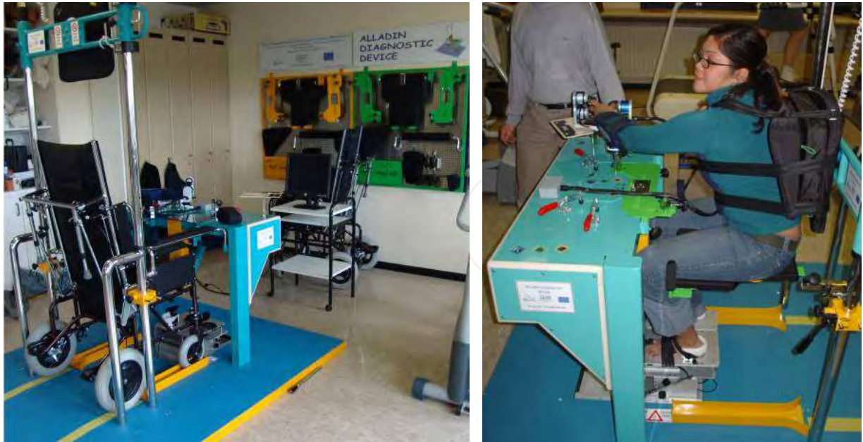
Fig. 5. The ALLADIN mechatronic platform for functional assessment of post-stroke subjects
