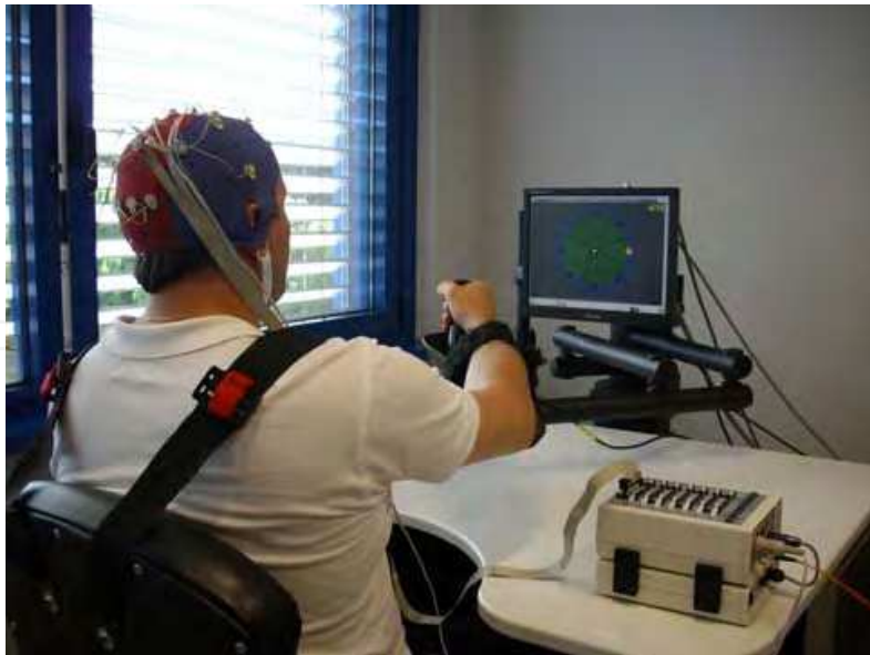
Fig. 2. A subject during the the robotic therapy using the MIT-Manus and recording of EEG signals for the functional assessment
