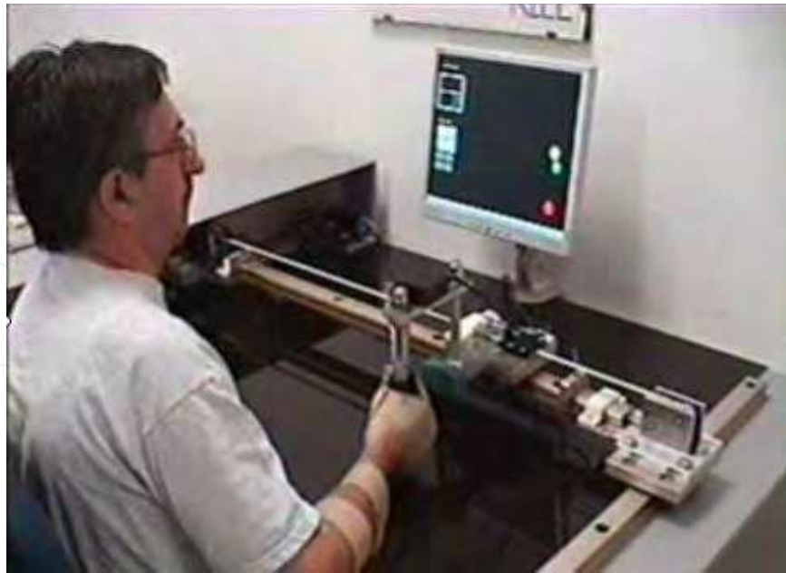
Fig. 3. The “MEMOS” system: a mechatronic system for the upper limb rehabilitation
