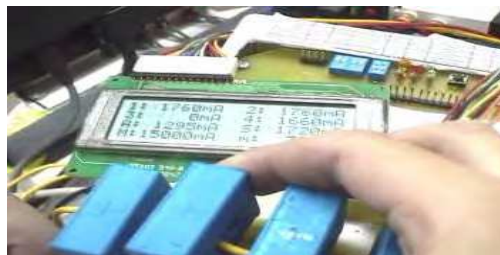
Fig. 13. The current sensor #2 and #4 are wrong
