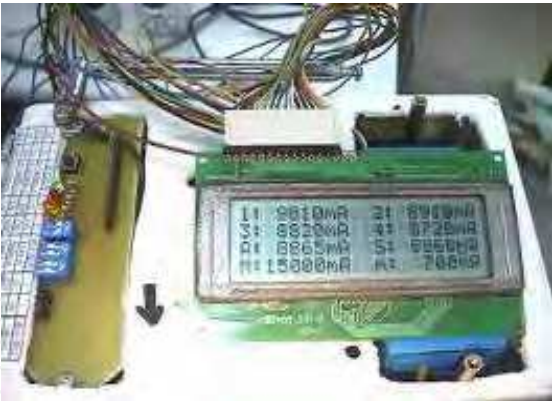
Fig. 4. The prototype of the power detection module
