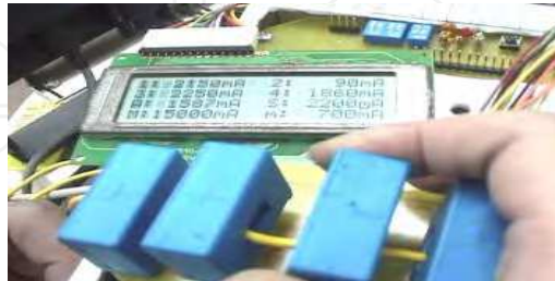
Fig. 13. The current sensor #2 and #4 are wrong
