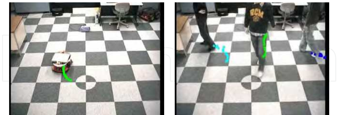
Fig. 5. Examples of mobile robot tracking and multiple people tracking using three laser range finders. The tracking results obtained in a position server mentioned below are overlaid on video images.
