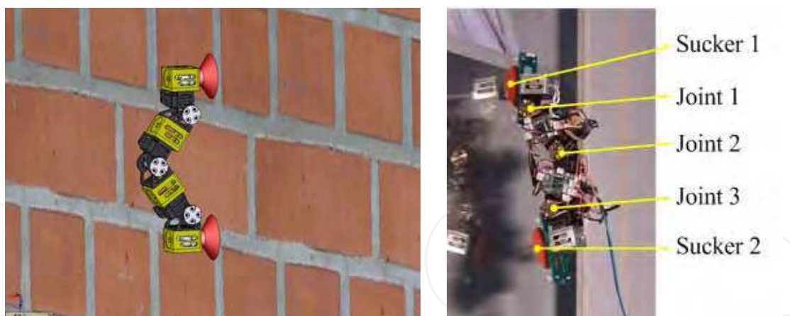
Fig. 4. Robotic inchworm design in CAD and real prototype
