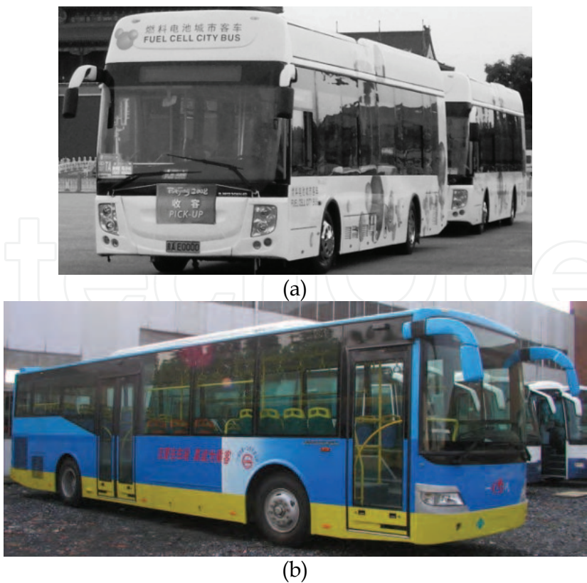
Fig. 1. (a) Fuel cell city bus (b) Diesel engine series hybrid city bus
