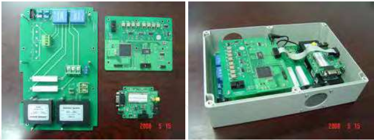
Fig. 12. Implementation of the sensing, processing and communication unit
