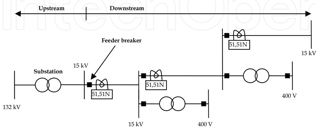
Fig. 1. Overcurrent relays applied to radial distribution network
