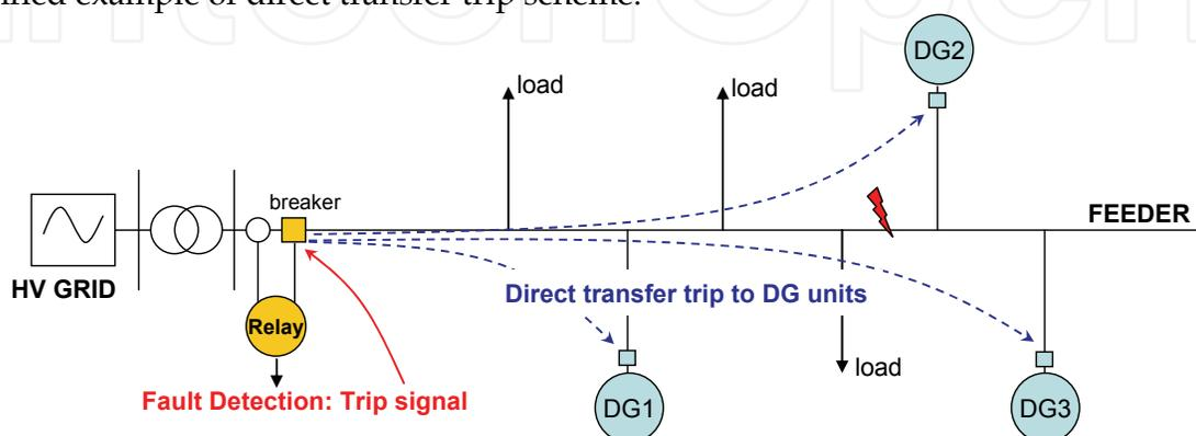
Fig. 7. Example of direct transfer trip scheme
