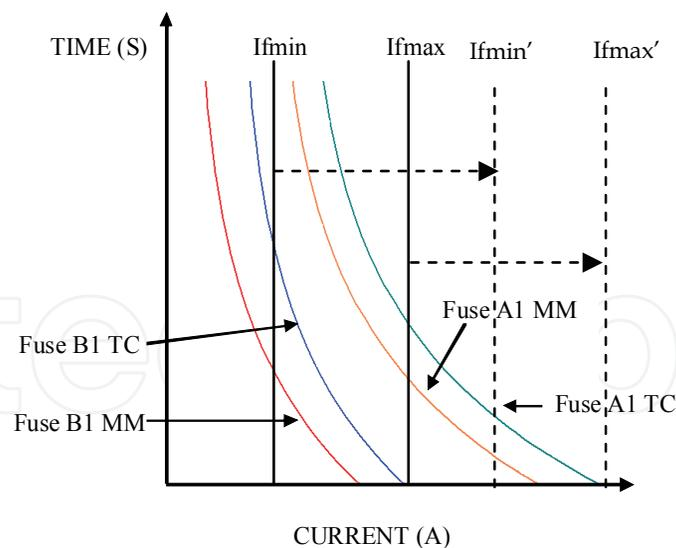
Fig. 4. Coordination graphic of fuses A1 and B1
