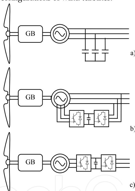
Fig. 8. Wind turbine configuration
