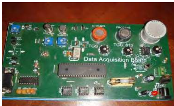
Fig. 1-b. Electronic nose of gas detection without chamber
