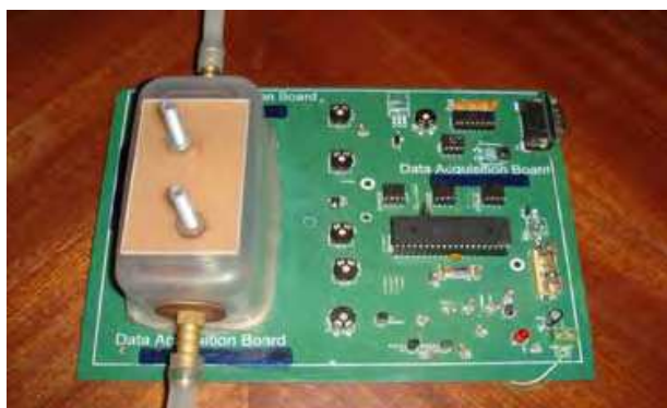
Fig. 1-a. Electronic nose of gas detection with chamber
