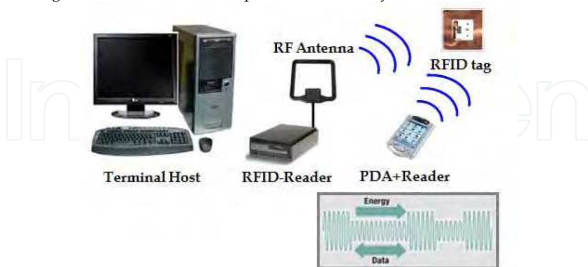
Fig. 2. Usual components of a RFID system
