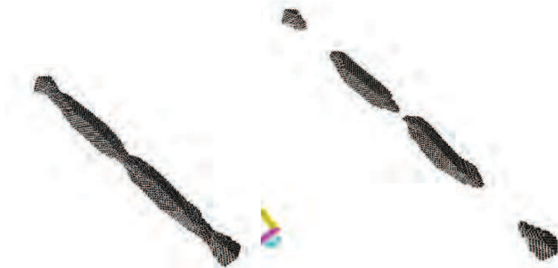
Fig. 5. Tensile deformation and failure of 5×5×60 Nickel nanowires; strain rate=1.67×10 10 (s -1 )
