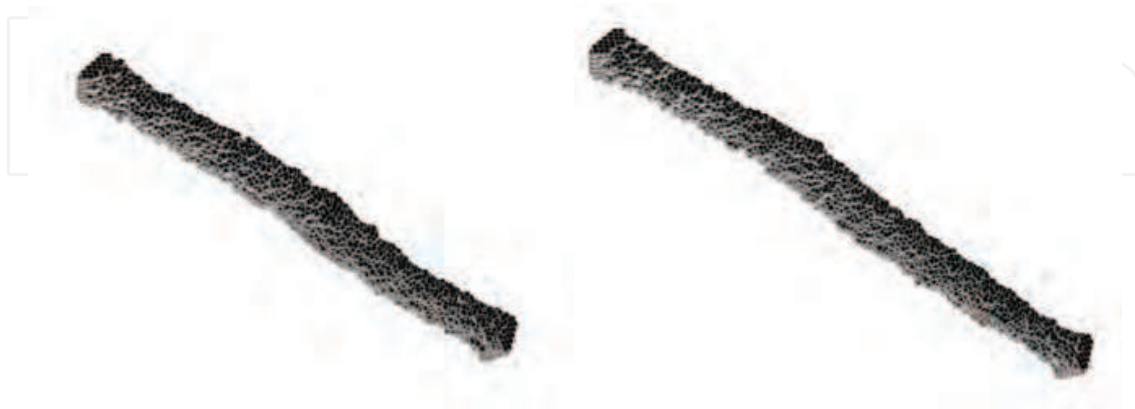
Fig. 9. Deformation configuration of 5×5×60 Nickel nanowire at T=1600K
