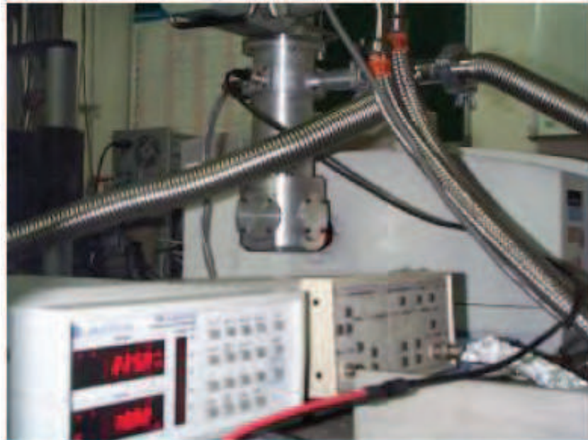
Fig. 9. The physical FTIR and cryostat systems for temperature-dependent photoresponse measurement
